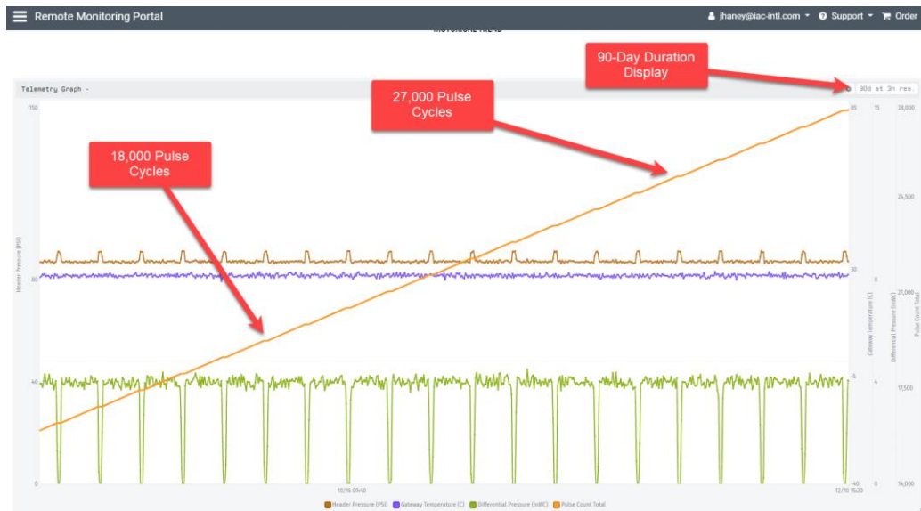
Fig. 4 – Example of tracking pulse valve activation count through filter life cycle
