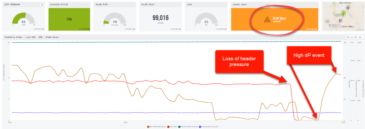
Fig. 8 – Onscreen representation of high dP even seen in connected web portal
